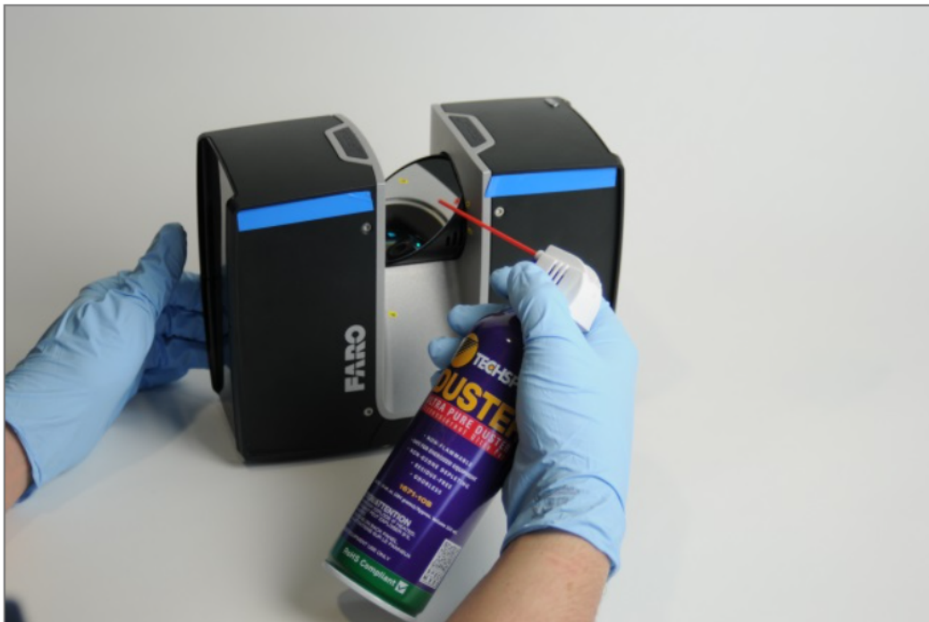
Figure 10-10 Dry pre-cleaning by compressed air or duster cleaning spray
