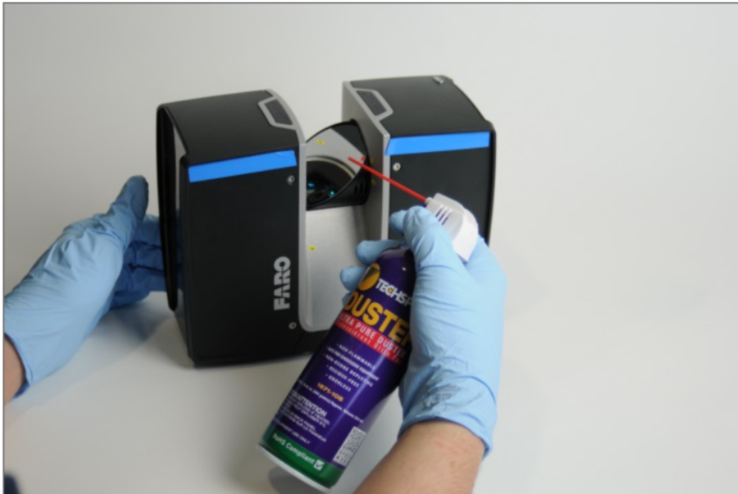
Figure 10-1 Dry pre-cleaning with compressed air or duster cleaning spray
