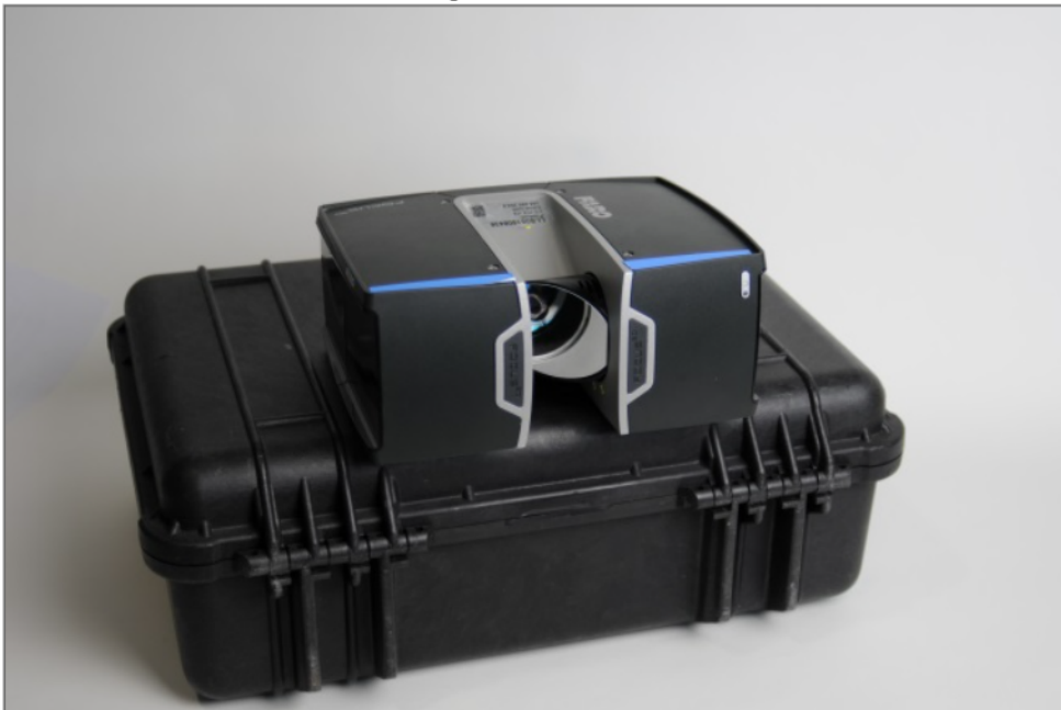
Figure 10-11 Transport box with laser scanner turned and laid on top, with the mirror module facing outwards
