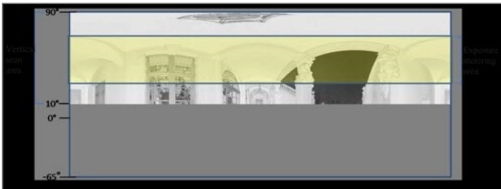
Figure 8-14 Exposure metering area for a limited vertical scan area set to e.g., 10^\circ to 90^\circ
