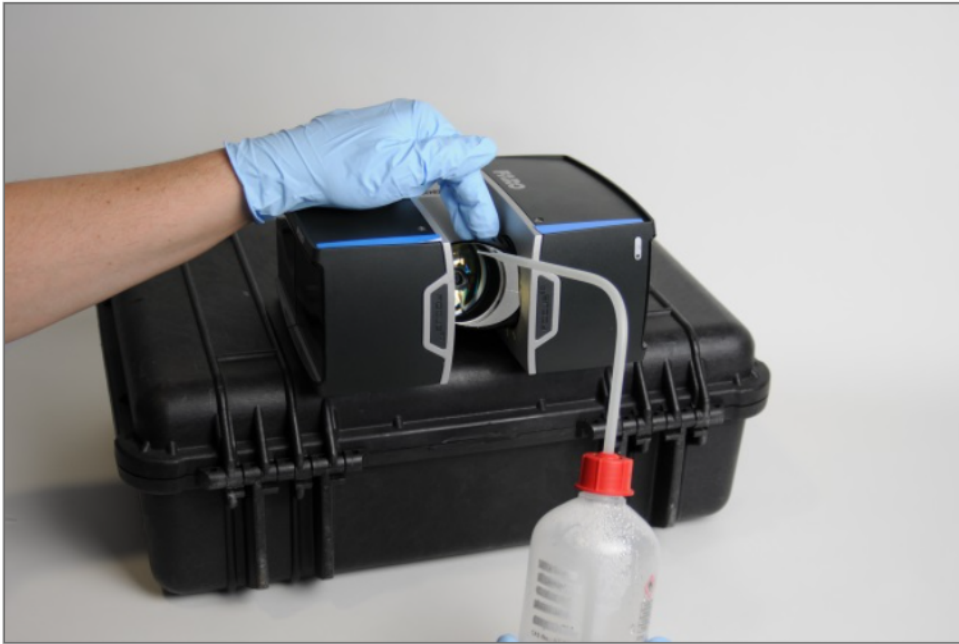
Figure 10-13 Cleaning mirror module or sensor cover
