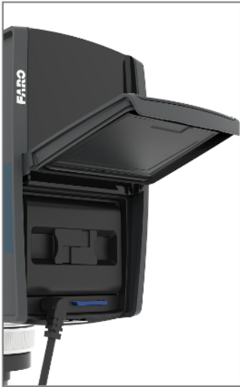
Figure 7-2 Power Supply connected to FARO Laser Scanner
