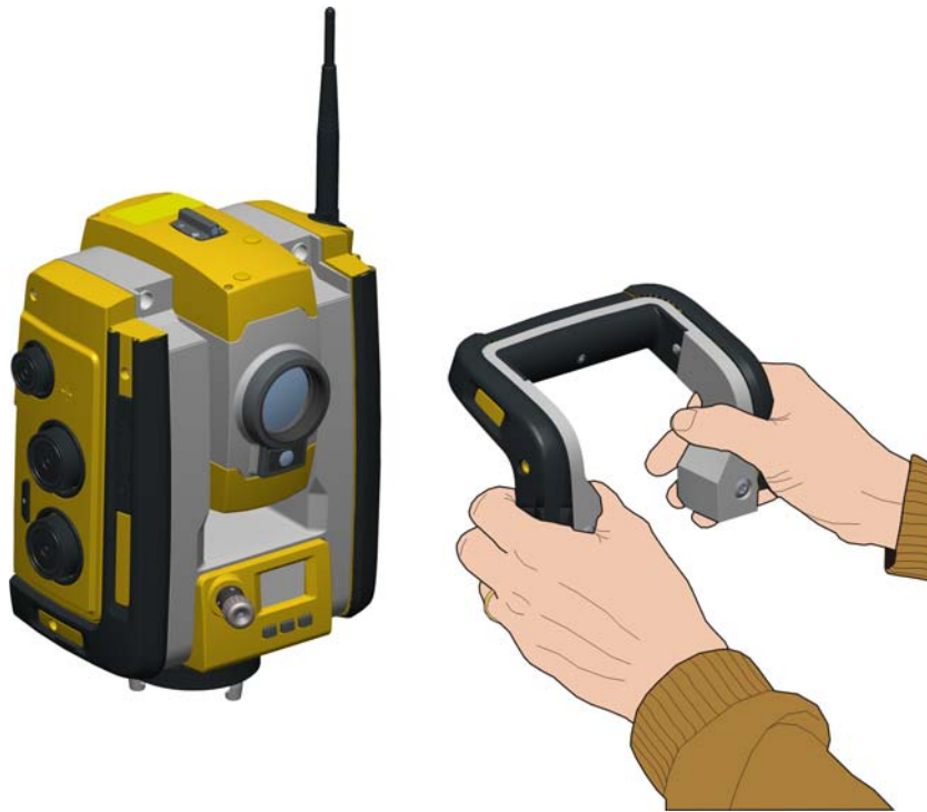
Figure 4.35 Detaching the Trimble SPSx20 Total Station handle
