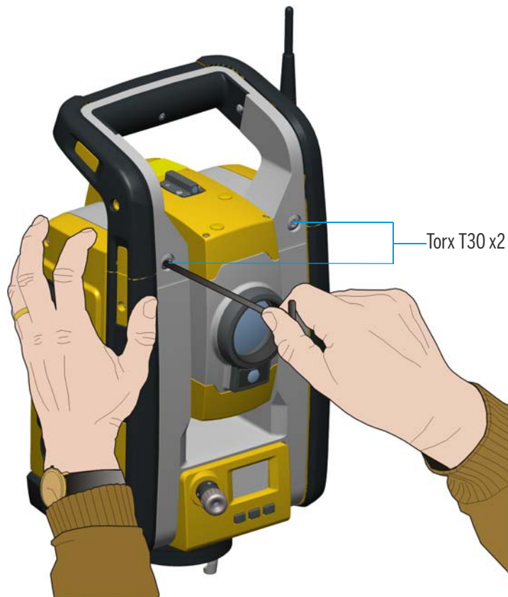
Figure 4.34 Removing the Trimble SPSx20 Total Station handle
